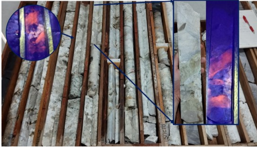
Figure 2 - DHAB-214 showing mineralization with large spodumene crystals identifiable under UV light.
