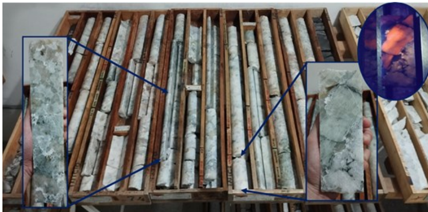
Figure 3 - DHAB-220 showing mineralization with large spodumene crystals identifiable under UV light.
