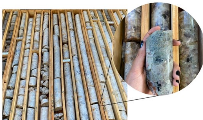
Figure 1 - Mineralized spodumene intersects with coarse, large crystals from DHAB-290 in Anitta 4
