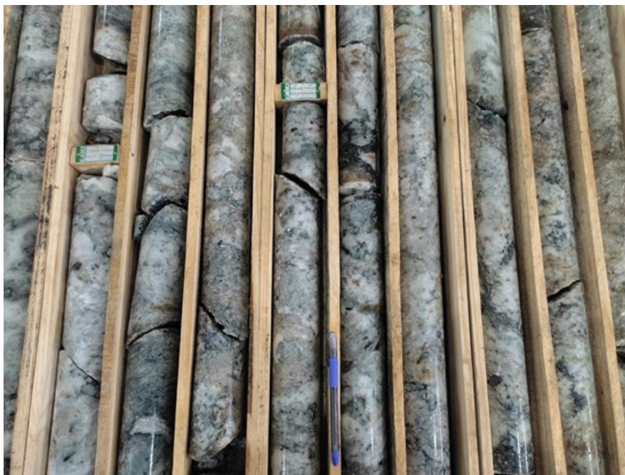
Figure 1: Lithium-bearing spodumene cores from drill hole DHAB-162 (part of the 103.4m continuous intersect)
